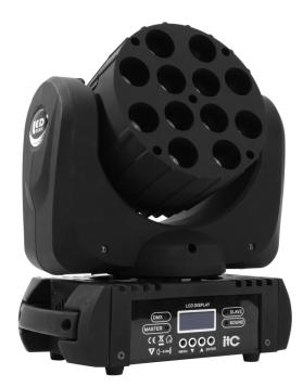
Feature: \* Dimming: 0-100% linear adjustment. \* Color mixing: RGBW stepless color mixing. \* Strobe: 1-25 times/sec (conventional strobe, thunder strobe, random strobe, suddenly dark gradually brighter strobe, suddenly bright gradually darker strobe. 1-20 times/see (see 12 strobe). \* Scan range: X-axis 540 degrees; Y-axis 270 degrees; fast running speed, mute design, and adjustable speed. \* Scanning fine-tuning: X/Y axis 16BIT scanning subdivision for accurate positioning.
